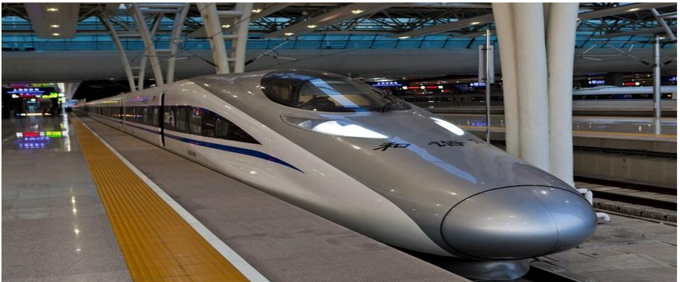
Harmony CRH 380E - The Harmony is an electric high speed train which travels between Shanghai and Beijing. It took four and a half years to build the tracks which cost in excess of $17 billion. It is the world's second fastest train cutting down the travel time from 10 hours to less than 3 hours travelling at speeds of 380 km/h. The design uses a greatly improved vibration system and improved air tightness for passenger comfort. Advanced sound absorbing materials and insulation are used for the carriages.
