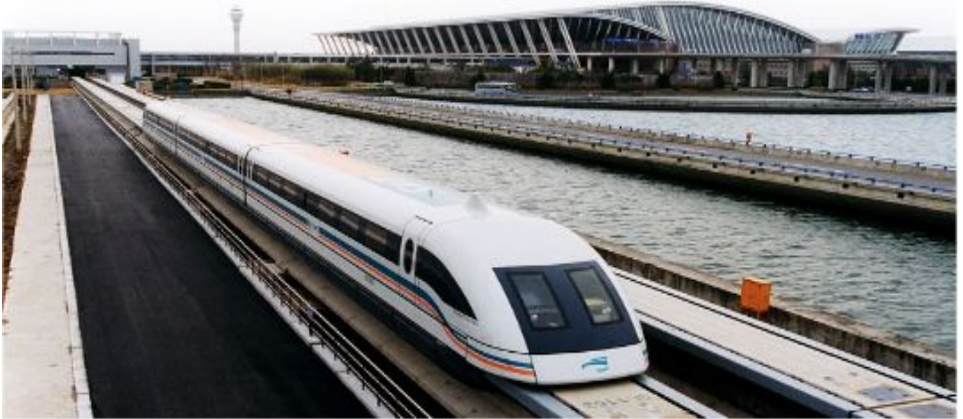
Shanghai Maglev - The journey from Shanghai to Shanghai Airport takes only 7 minutes and 20 seconds thanks to the incredible maglev trains. This train uses magnets to levitate above the tracks which reduce friction allowing the train to reach speeds of 430 km/h. Following a serious accident in Germany in 2012, the Chinese authorities have reduced the speed at which the train runs to 298 km.
